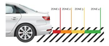
Activates when reverse gear is engaged - one initial beep
